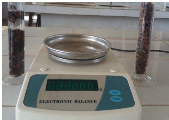
Figure 3: Solid Density Apparatus: Fractional Cylinder and Weighing Balance
